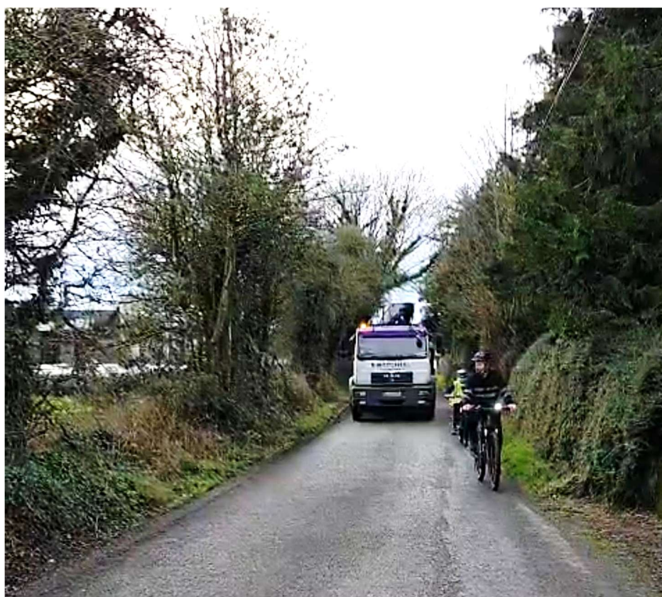
Figure 4.3 - This image shows cyclist and vehicle interaction on a constrained section of the L7108/L7109 corridor, highlighting the narrow carriageway, limited verge space and exposure of vulnerable road users.
